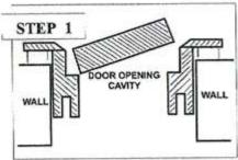
Fit SECTION 1 into the wall cavity. Level the opening Head and Style (and Door) and fix both jamb styles temporarily.
