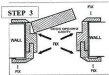
Check that the Door is both opening and closing properly and is balanced. Once complete, fix permanently.
