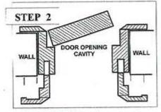
Fit SECTION 2 into the groove in the back of SECTION 1 and fix temporarily.
